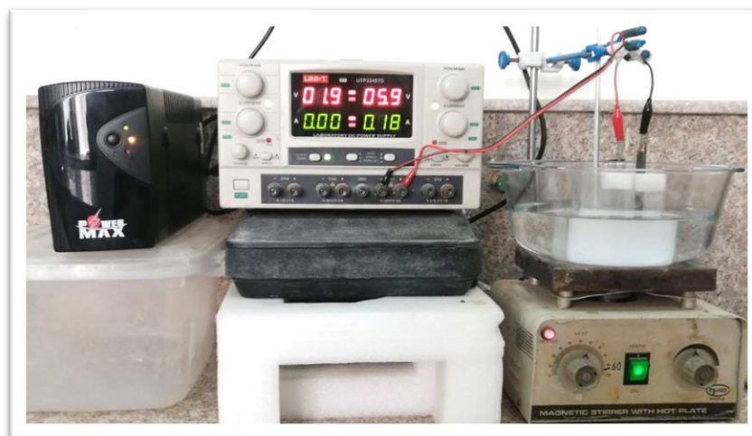
Figure 1. Electrochemical preparation of zinc oxide (NPs)
