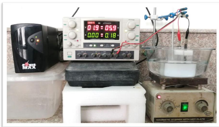
Figure 1. Electrochemical preparation of zinc oxide (NPs)
